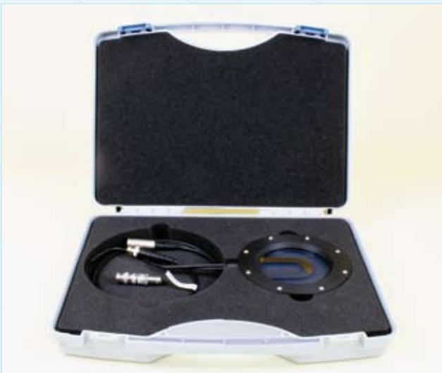
In order to operate the hydrophone without using the UHC-80 hydrophone controller, a separate power supply unit is available. The measured values are recorded by means of a suitable oscilloscope. In order to connect the membrane hydrophone to an oscilloscope, a suitable broadband in-line network terminator (50 Ohm) is available.
